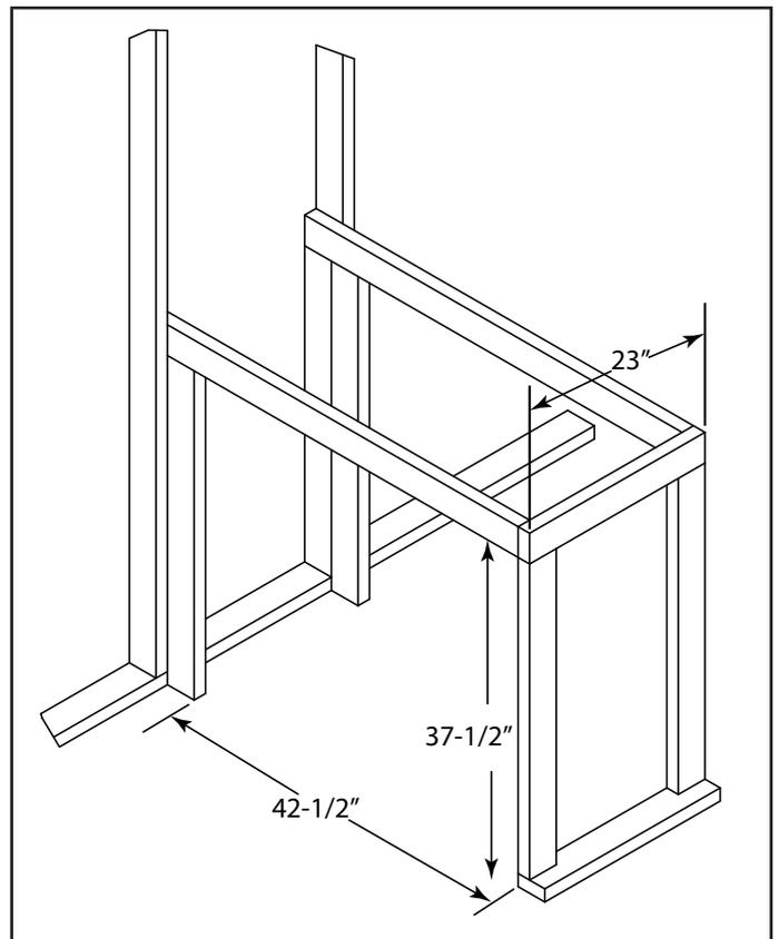
Figure 4.3 Framing Specifications
