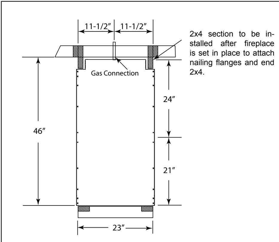
Figure 4.2 Top View of Framing Specifications
