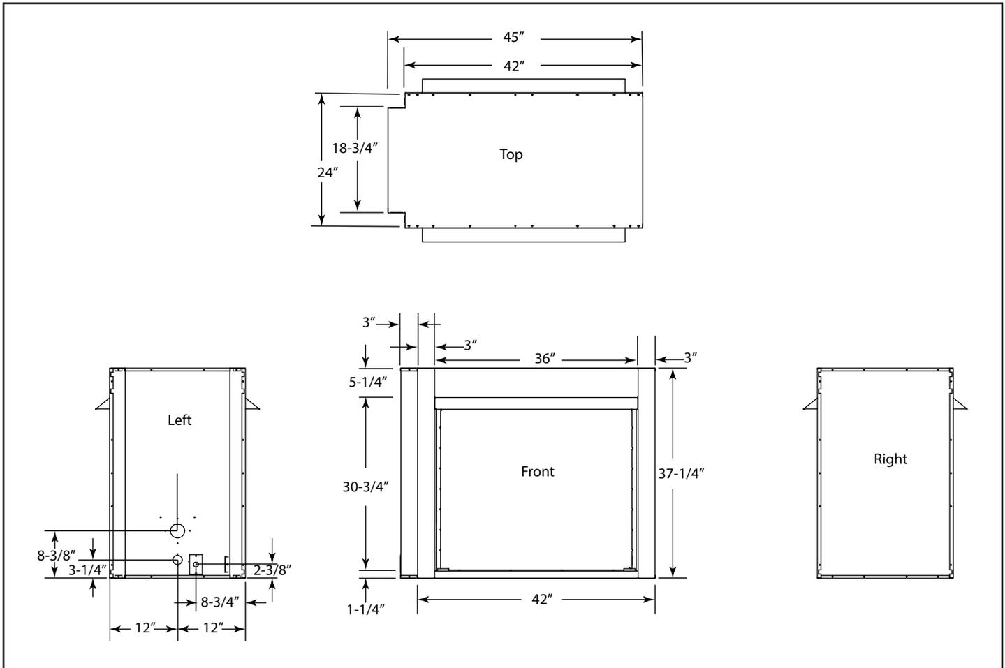
Figure 4.1 Framing Dimensions
