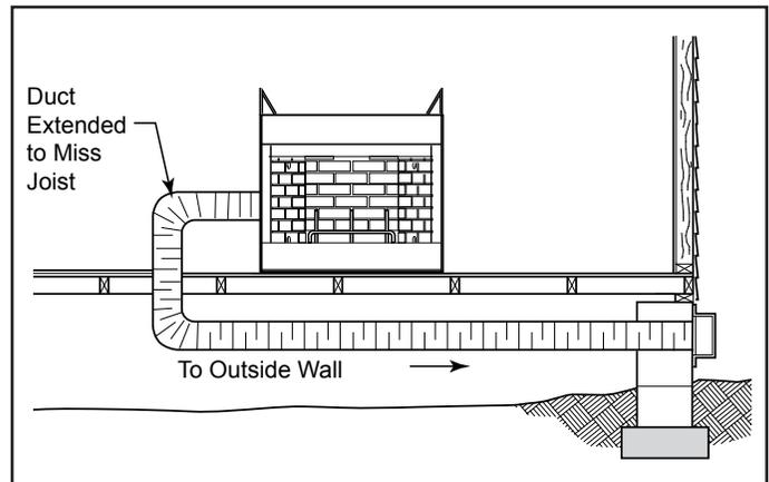
Figure 8.3 Installation Above Basement or Crawl Space
