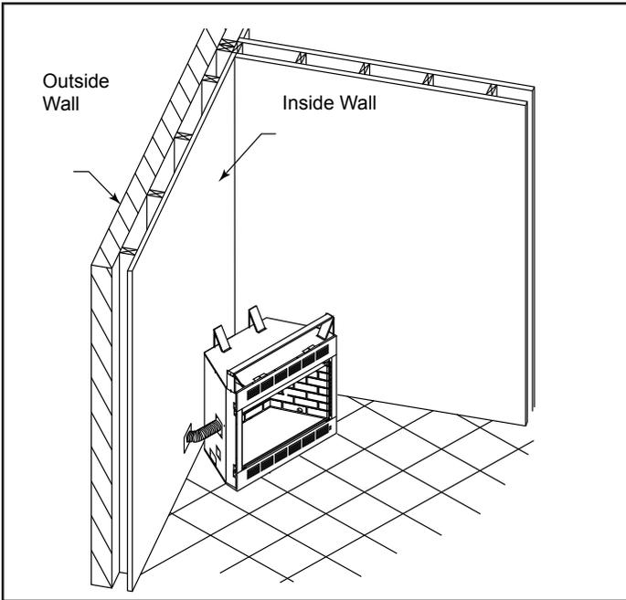
Figure 8.4 45° Corner Installation on Slab Floor
